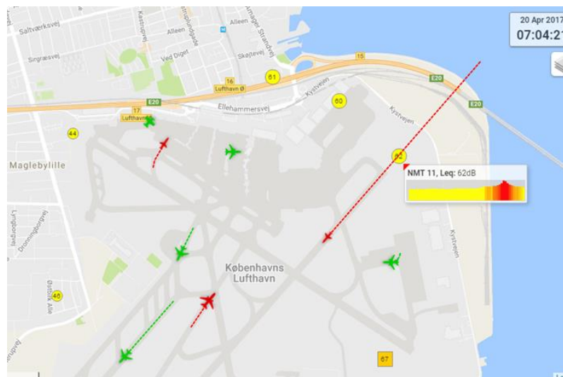
Figure 25: Copenhagen’s WebTrak system showing a noise event (in red) as registered by a noise monitor
